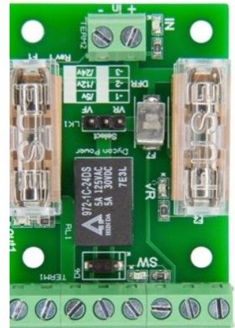
The DFR-1-12 12VDC and DFR-1-24 24VDC relay modules are ideal for use as fire relays on access control systems
